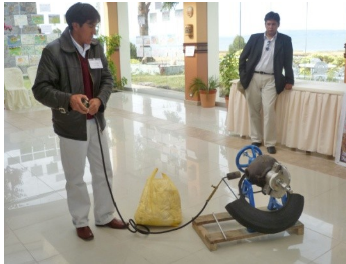
Figure 10. Popping machine prototype similar to the ones found locally that reduces lead values in the product processed.
